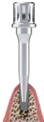
Fig.12: The fixture remover rotates counterclockwise to remove the implant from the bone in the direction of the grooves it fits into.
