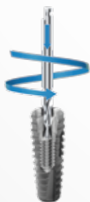
Fig.6: The appropriate reverse drill is selected. Drilling is carried out in intervals, counterclockwise, at 600-700 rpm.
